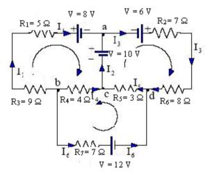
What are the I<sub>1</sub>, I<sub>2</sub>, I<sub>3</sub>, I<sub>4</sub>, I<sub>5</sub>, I<sub>6</sub> current values in the many loop electric circuit figures?
